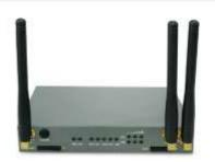
The Galgus Industrial grade 3/4G router dual SIM with WIFI a/b/g/n the best and simplest option for professional communications requiring an expanded 3/4G connectivity with double WAN data rates and 4 LAN ports, with an extended grade in its environmental conditions and working mode.
