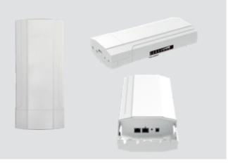
Galgus OC400 delivers the most advanced wireless communications features up to **1000mW high power outdoor 802.11ac environment.**
