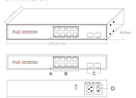
A.Working indicator C.2\*Gigabit SFP ports
