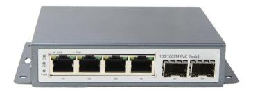
The G-SW-4P2S series is a full gigabit PoE fiber switch. It has 4\*10/100/1000M RJ45 ports and 2\*1000M SFP slot ports. Port 1-4 can support IEEE 802.3af/at standard PoE power supply. single port PoE power reaches 30W, and the maximum PoE output power is 65W (at-110W).
