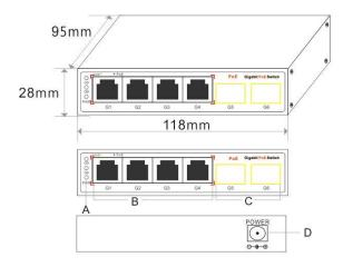
A. Power indicator C. 2\*1000M uplink SFP ports B.4\*10/100/1000M PoE ports D.DC power port
