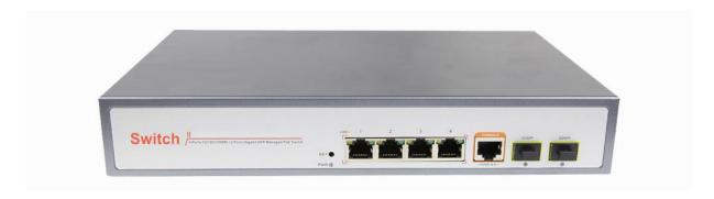
The G-SW-M4G2S is a full gigabit L2+ managed Ethernet fiber switch. It has 4\*10/100/1000Base-T RJ45 ports and 2\*100/1000Base-X SFP fiber slot ports. Each port can support wire-speed forwarding.
