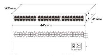
A. RJ45 PoE Output B. Ethernet RJ45 Input C. PoE Status Light D. AC 220V/50Hz Input
