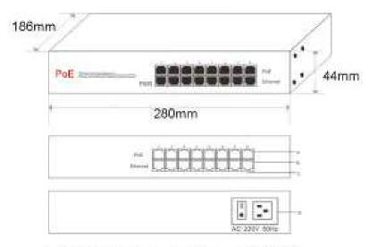
A. RJ45 PoE Output B. Ethernet RJ45 Input C. PoE Status Light D. AC 220V/50Hz Input
