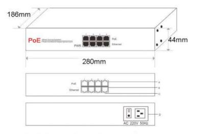
A. RJ45 PoE Output B. Ethernet RJ45 Input C. PoE Status Light D. AC 220V/50Hz Input
